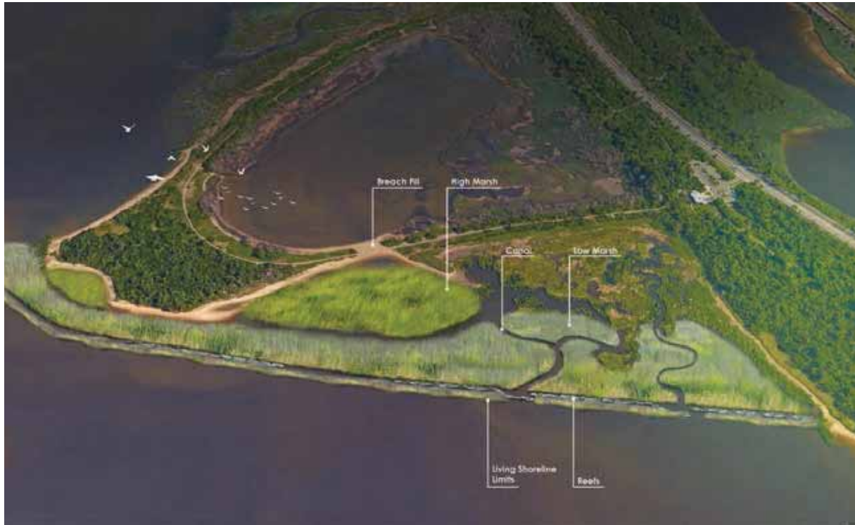
An aerial rendering of Jamaica Bay illustrates shoreline stabilization tactics in New York. Photo by Stantec
