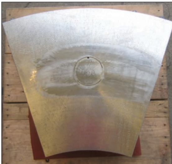
(i) Wiped thrust bearing shoe.
